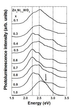
Figure 2. Photoluminescence of microcrystalline pure ZnWO<sub>4</sub> (x = 1) and the Zn<sub>x</sub>Ni<sub>1-x</sub>WO<sub>4</sub> solid solutions annealed at 800°C
