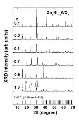
Figure 1. X-ray diffraction patterns of the microcrystalline  $ZnWO_4$  and  $Zn_xNi_{1-x}WO_4$  solid solutions annealed at  $800^{\circ}C$ . (Only a few patterns are shown for clarity).
